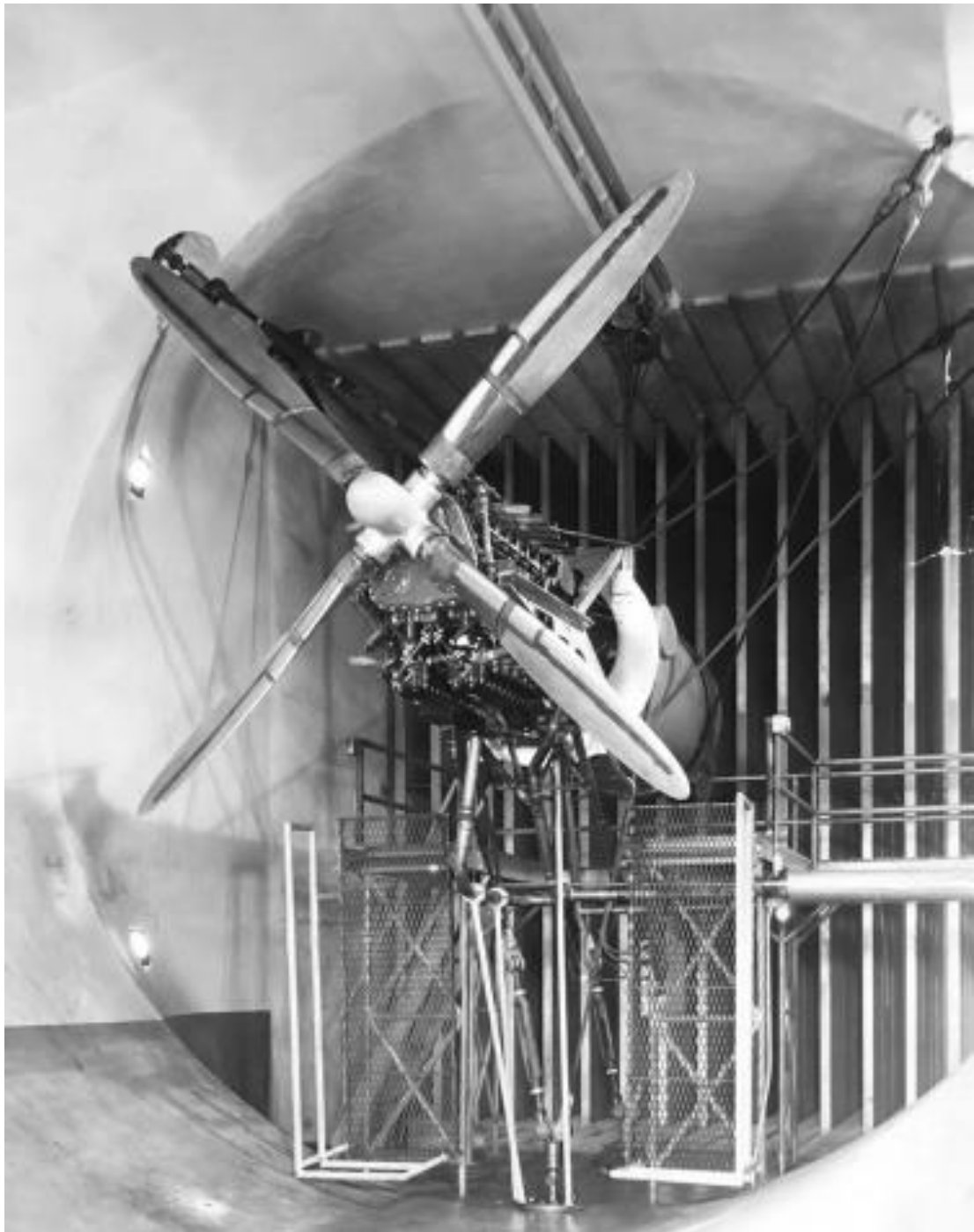
An XH-2470 mounted on a test stand with a tractor propeller. Installed in the XP-54 as a pusher; the blades on the XH-2470 had their angle reversed. Note the individual exhaust stacks.
