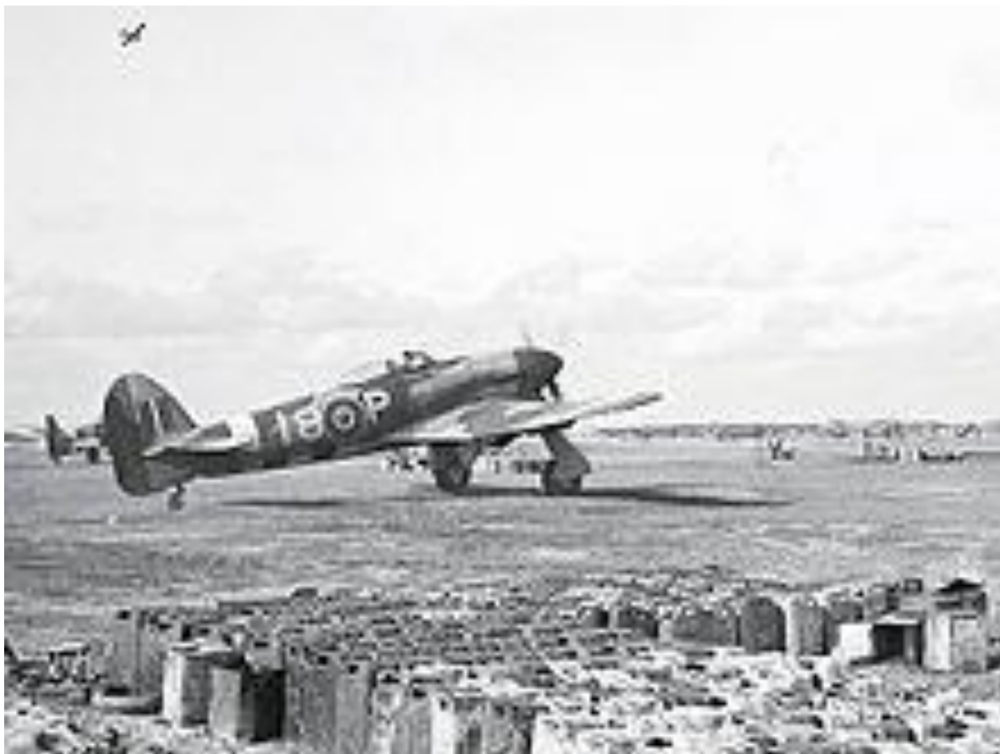
Late model Typhoon of 440 (RCAF) Squadron . Note the bomb rack under the wing. Rows of five-gallon jerrycans dominate the foreground
