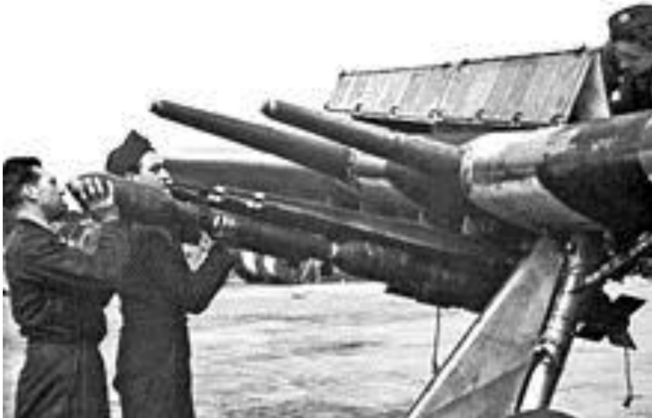
Armourers loading RP-3 rockets with 60 lb High Explosive heads onto steel Mk. I rails. The large hinged gun bay doors are open. The weathered Invasion stripes are on upper and lower wing surfaces, indicating this photo was taken some time in June 1944.
