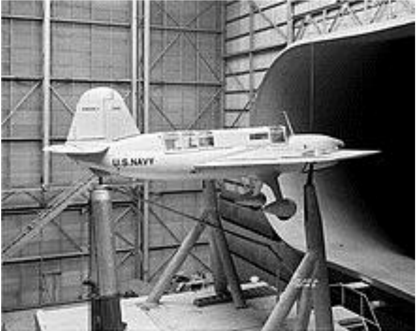
The Curtiss XSO3C in a wind tunnel, 1940
