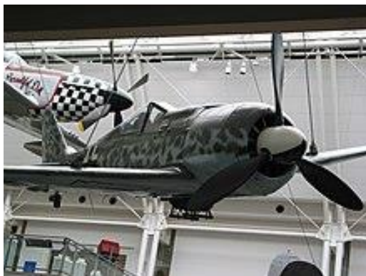
An Fw 190 A-8 (W-Nr:733682) at the Imperial War Museum showing faired-over gun ports and a belly-mounted ETC-501 bomb rack. This Fw 190 was used as the upper component for a Mistel flying bomb.
