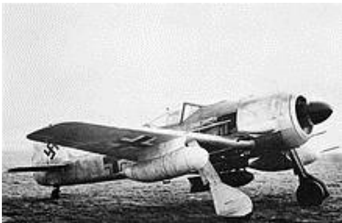
Fw 190 G-1 showing the ETC 250 bomb rack, carrying a 250 kg (550 lb) bomb, and the underwing 300 litre drop tanks on VTr-Ju 87 mounts.
