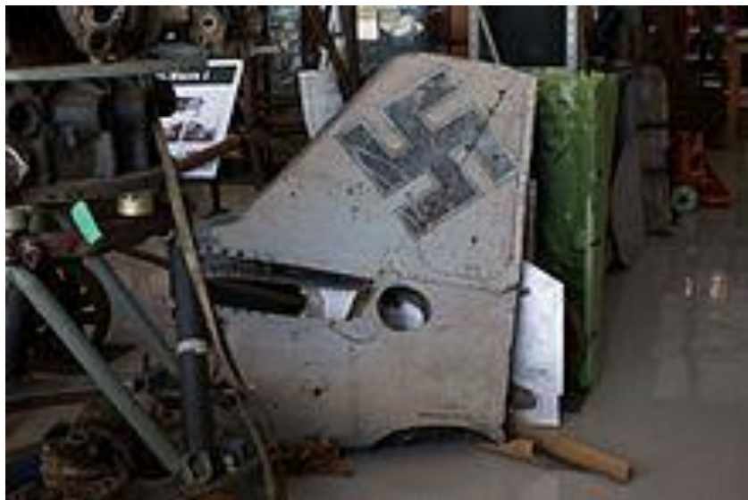
An Fw 190F's tailfin, showing the triangular hinged panel for access to the tailwheel retraction mechanics inside of it
