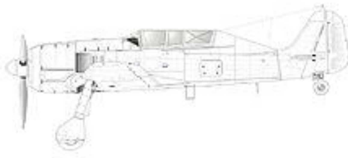
Fw 190 S-5 side view, showing the rear cockpit and extended canopy structure.
