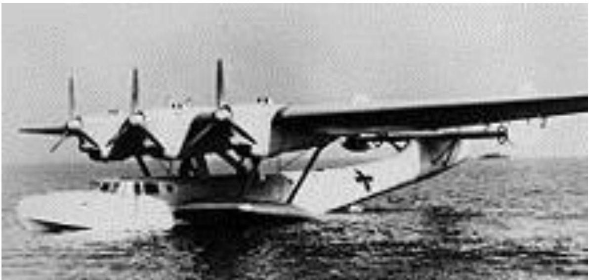
Diesel-powered Luftwaffe Do 24 V1 trials aircraft being used as an air-sea rescue aircraft
