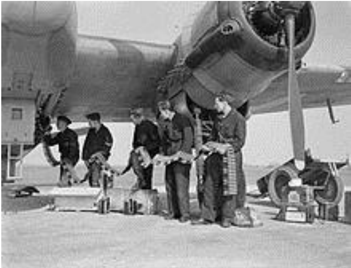
Ground crew loading ammunition for the cannon of an RAF Beaufighter Mk.VI night fighter
