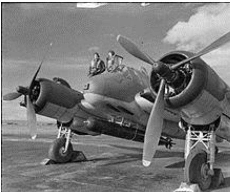
A Mk.VIC loaded with an 18-inch Mark XII torpedo
