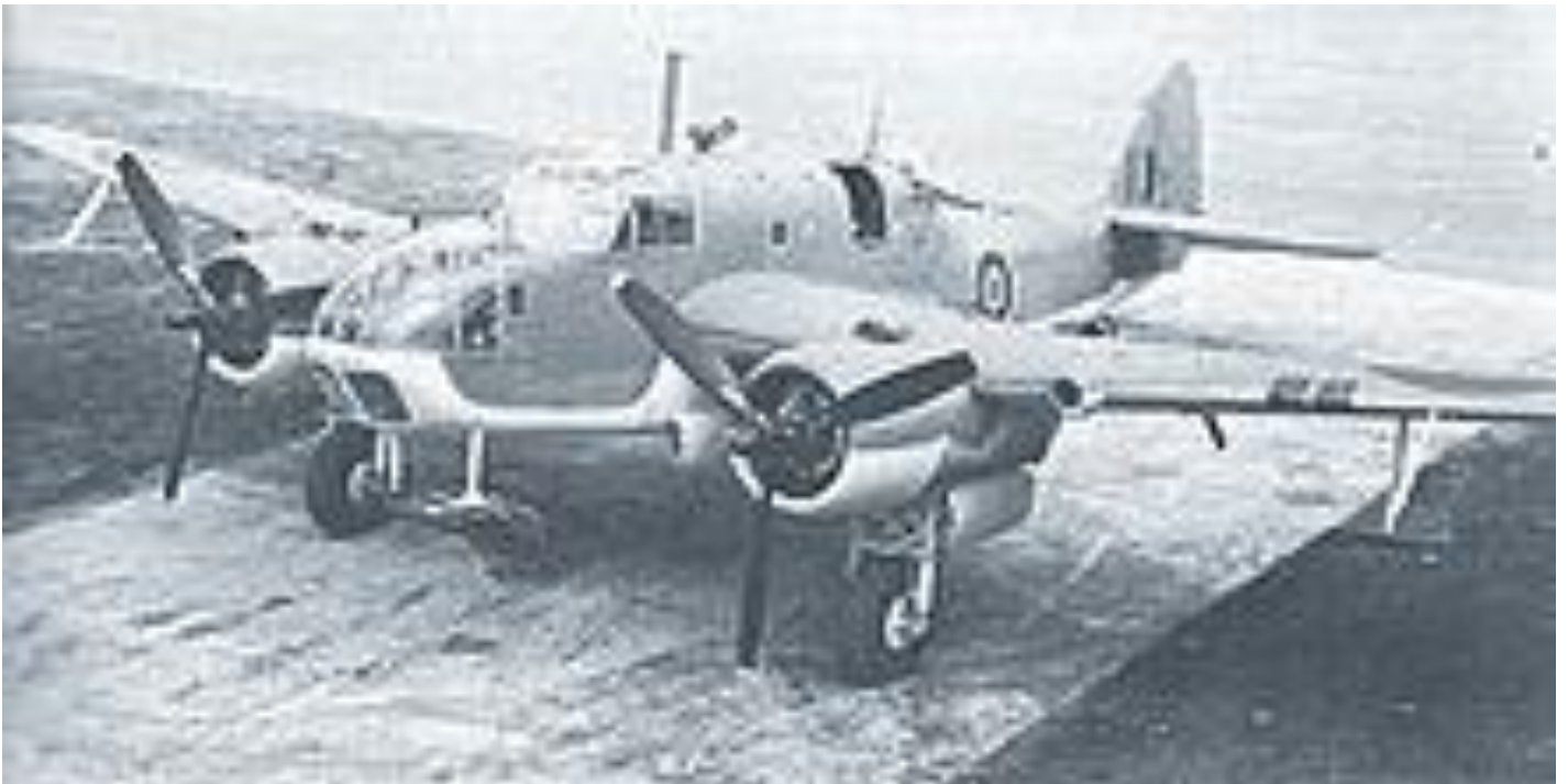
A new late-production Beaufort Mk.II at the Filton factory. ASV yagi aerials are under the nose and wings and the new DF loop is fitted. Muzzles of additional Vickers GO are visible in the front upper nose.
