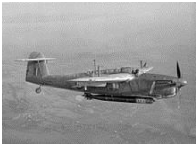
Barracuda Mk II carrying an 18-inch (46 cm) aerial torpedo . The ASV radar "Yagi" antennae are visible above the wings.
