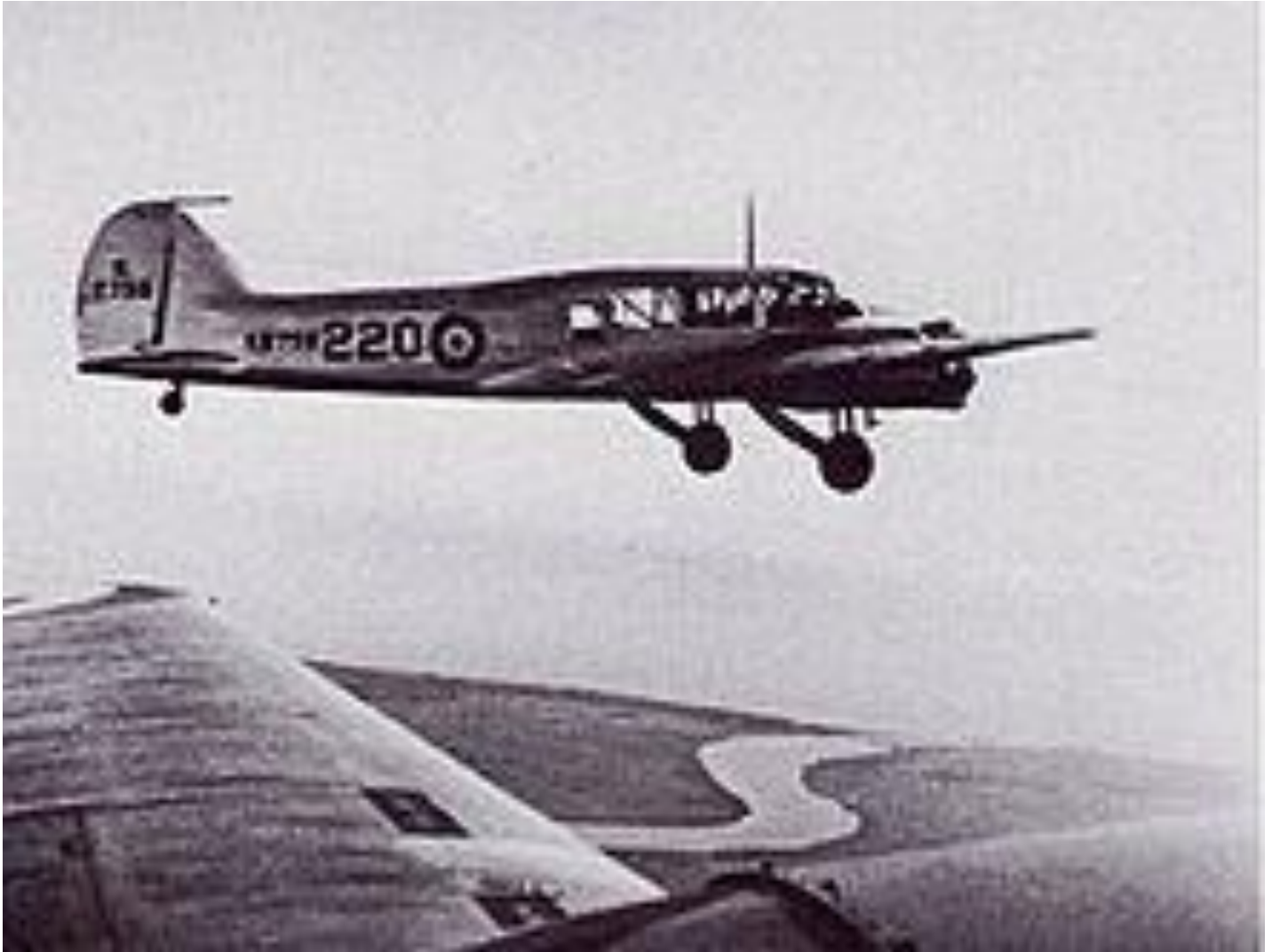
RAF Ansons conducting trials with airborne radar in 1937.
