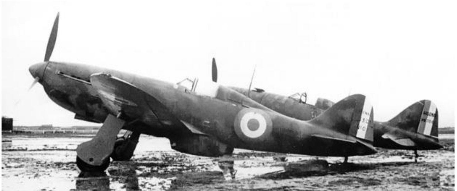
The VG 33 prototype sits complete with main gear doors on a muddy airfield. Many of the completed VG 33s, like the second aircraft in the image, were finished without gear doors.
