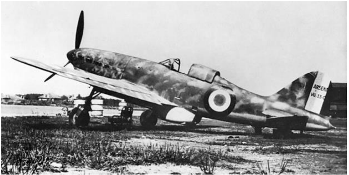
A completed VG 33 without gear doors seen at Toulouse-Blagnac airport in June 1940. Note the radiator housing under the fuselage.
