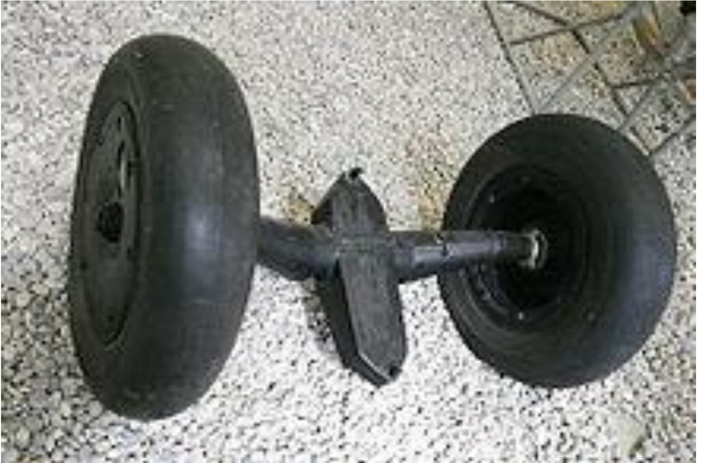
Me 163B's unsprung jettisonable main gear "dolly" unit
