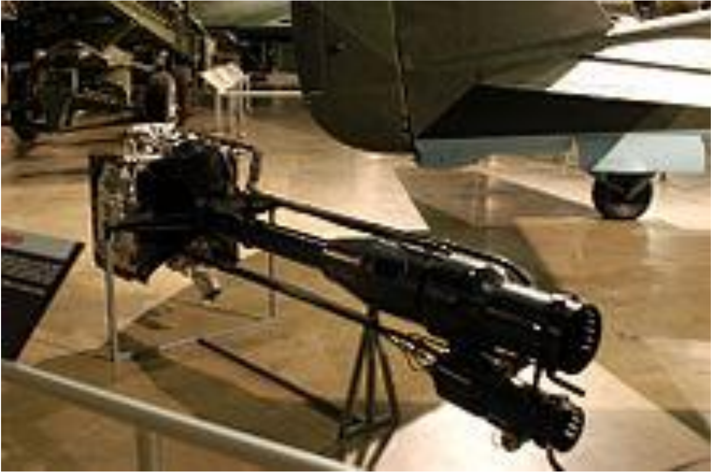
A preserved HWK 109-509B "cruiser" twin-chamber rocket motor ( National Museum of the United States Air Force )
