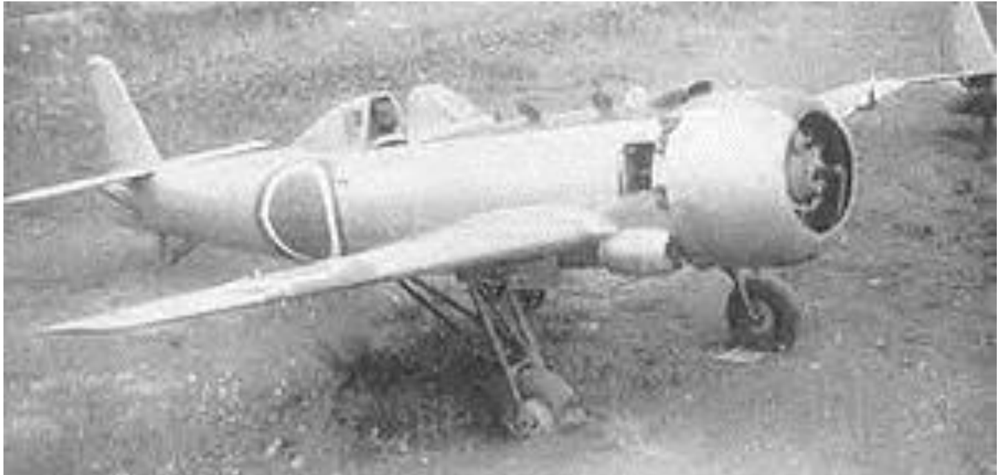
A Ki-115 shortly after the war. Propellers were removed to prevent flight. [7]
