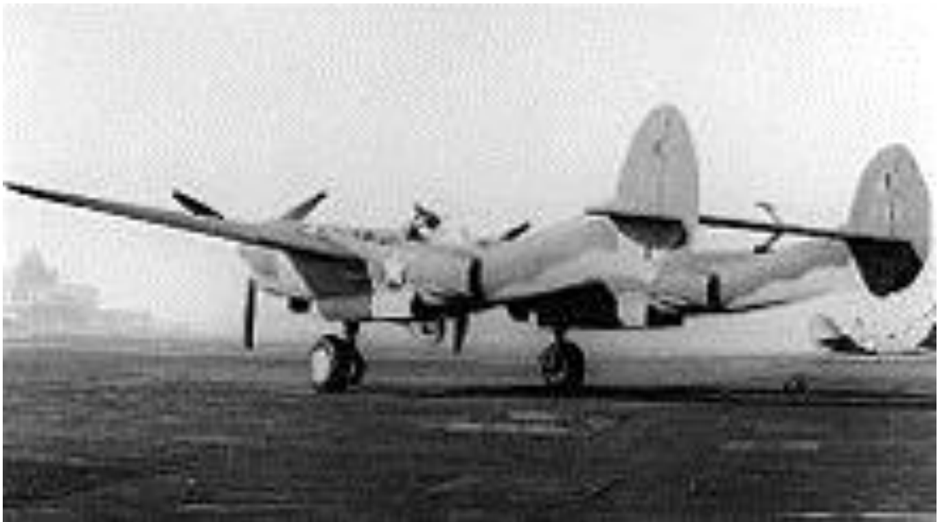
P-38E testbed 41-1986 shown with second version of upswept tail designed to keep tail out of water upon takeoff for a proposed twin-float variant
