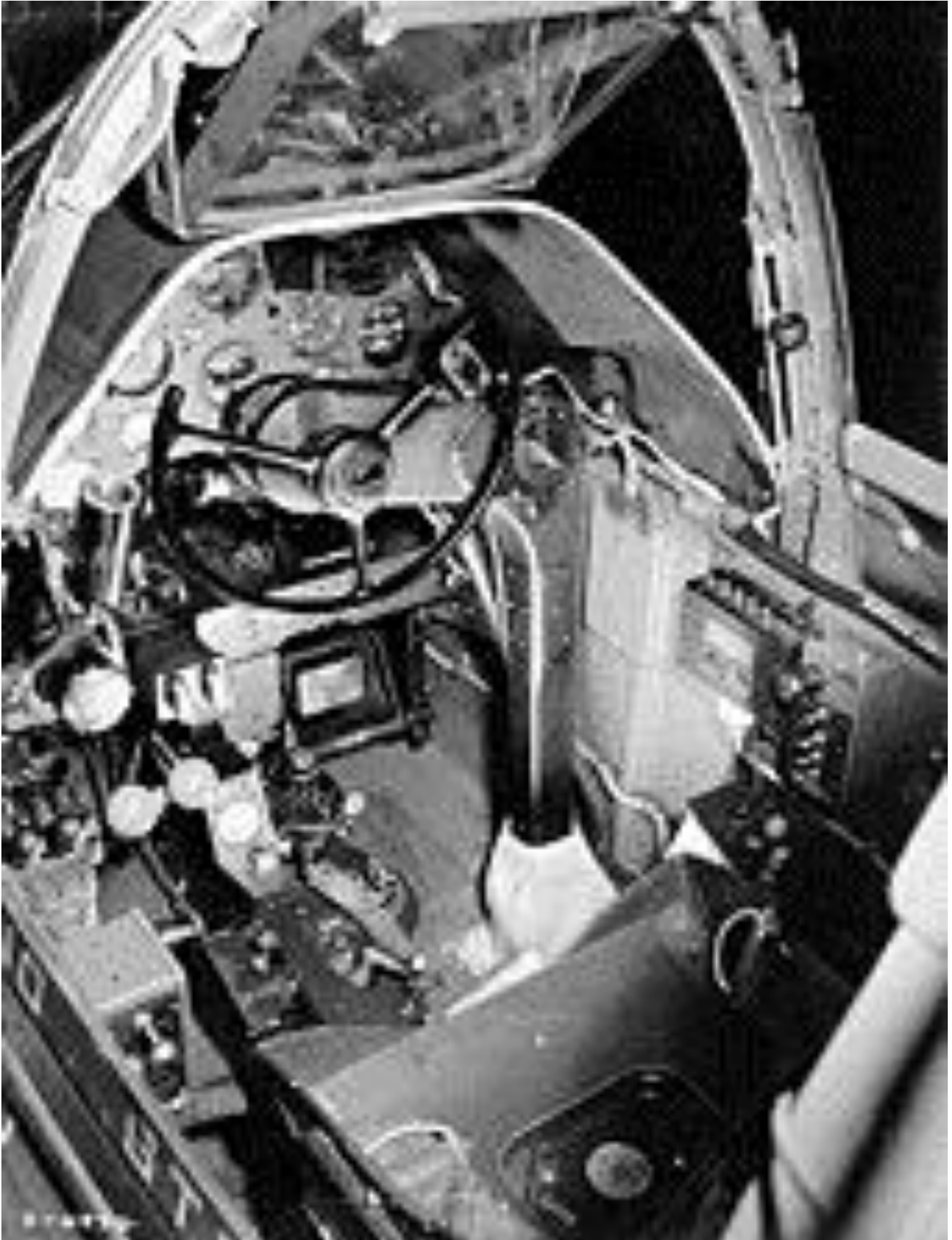
The P-38 was flown with a yoke, rather than the more-usual stick.
