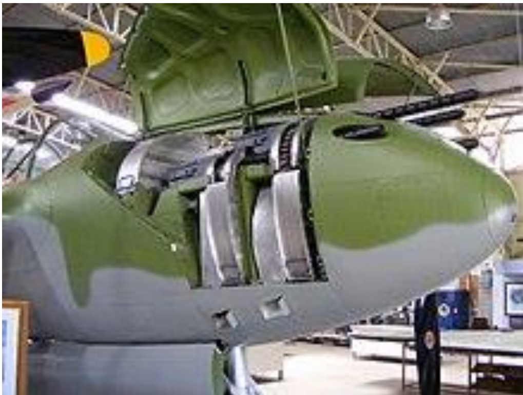
M2 machine gun armament in the nose of the P-38
