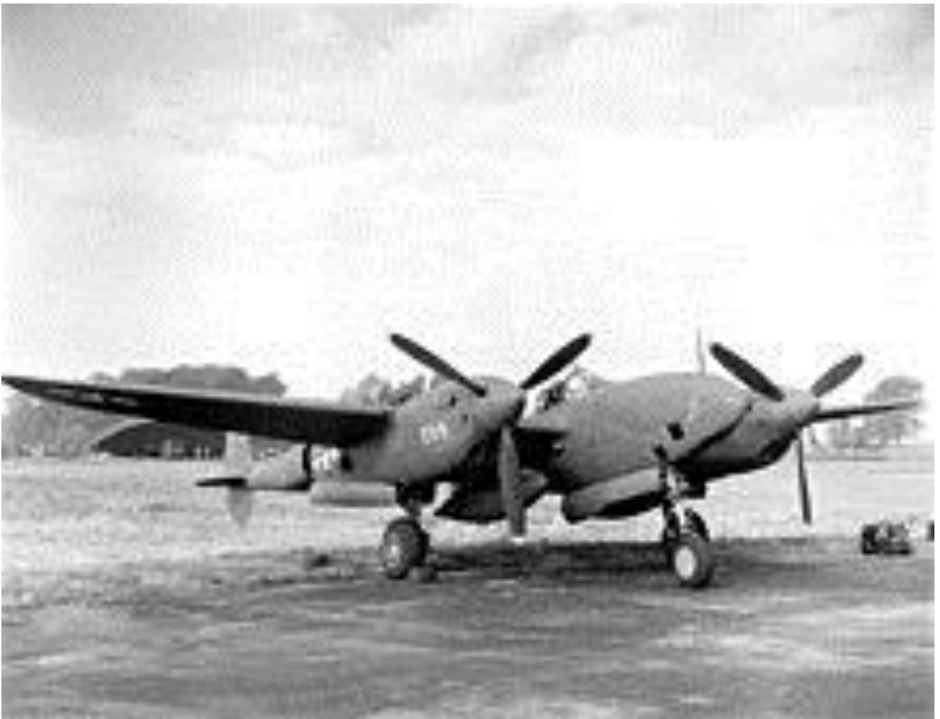
F-5A Lightning of the 7th Photo Group, 8th Air Force based at Mount Farm : The national insignia was bordered in red with overall finish in synthetic haze.
