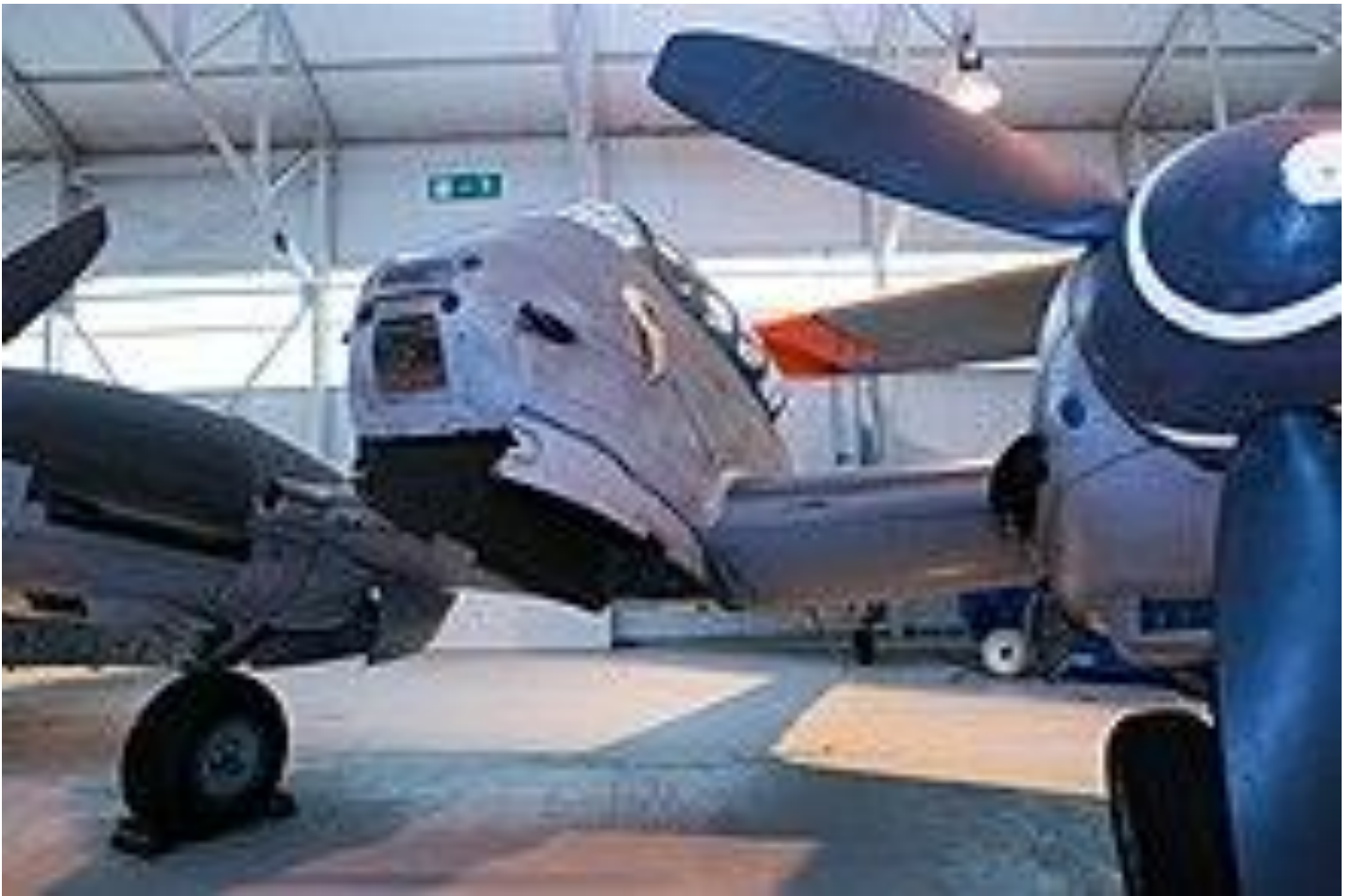
The RAF Museum's Me 410, with the doors of its nose bomb-bay open, 2016
