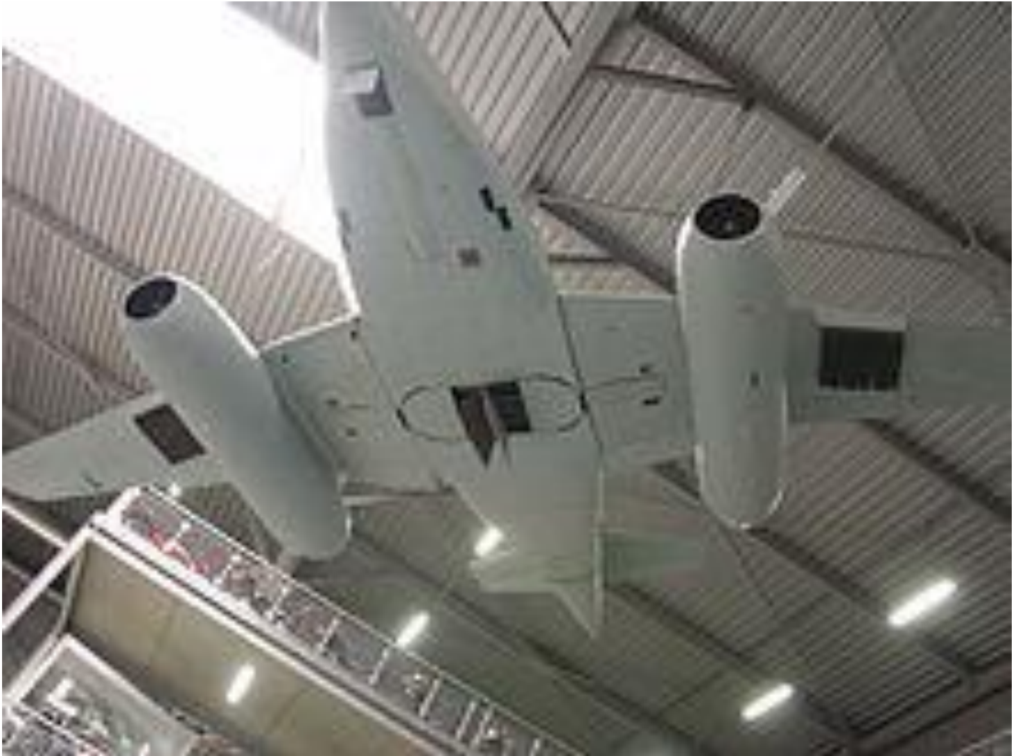
Mock-up of an Me 262A-1a/R7 with R4M underwing rocket racks on display at the Technikmuseum Speyer , Germany
