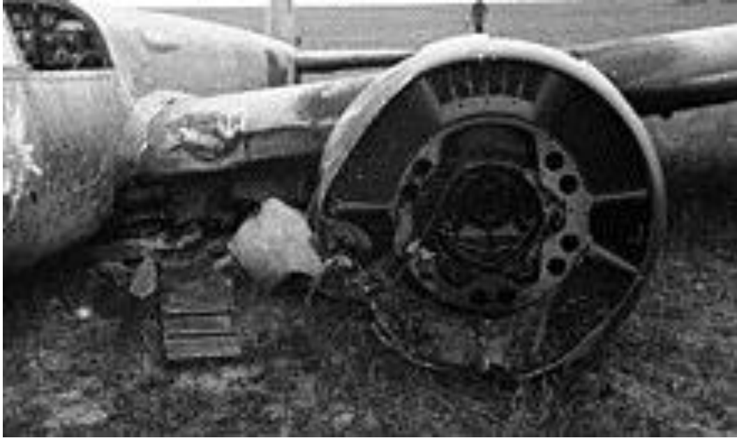
Annular radiator on a wrecked Ju 88
