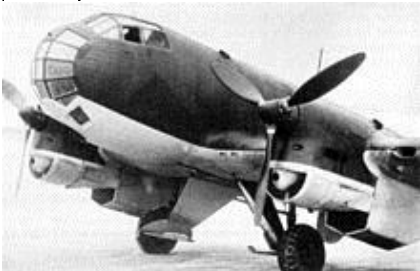
A Ju 86P high- altitude reconnaissance aircraft , with Jumo 207 turbocharged diesel powerplants.
