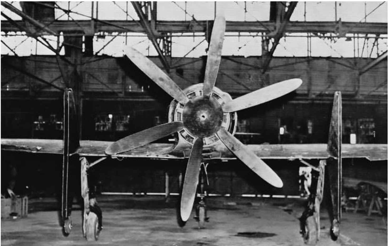
Rear view of the J7W1 showing its six-blade propeller and the engine's 12-blade cooling fan in the rear of the cowling. The exhaust augments outlet can be seen on the bottom of the cowling. Note the rudders extending the entire height of the vertical stabilizers.
