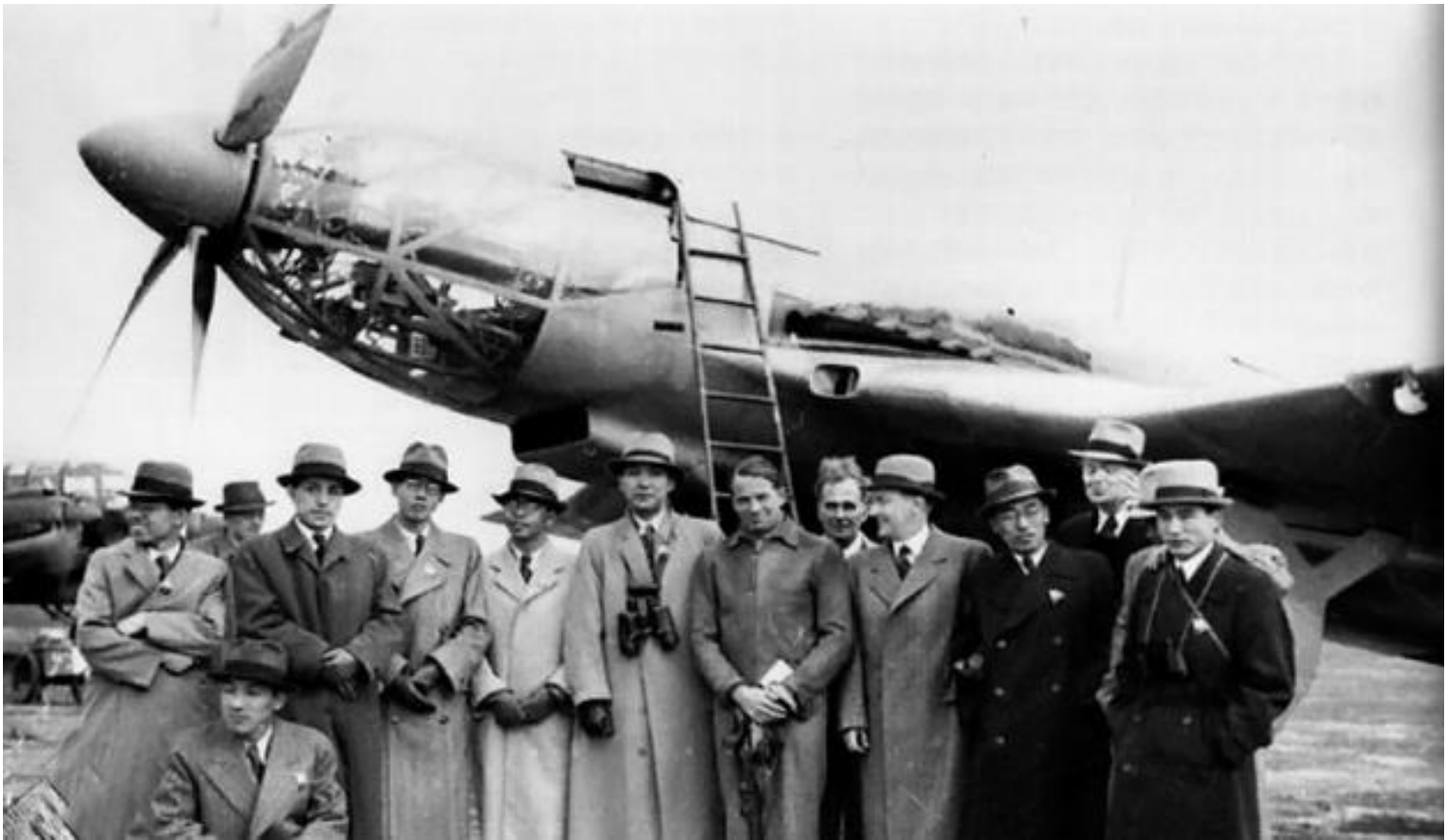
The Heinkel He 119 with the Japanese Naval delegation. The sliding roof panel for the pilot's cockpit access can clearly be seen. Note the differences with the wing root intake and lower lip of the radiator compared to the D-ASKR aircraft.
