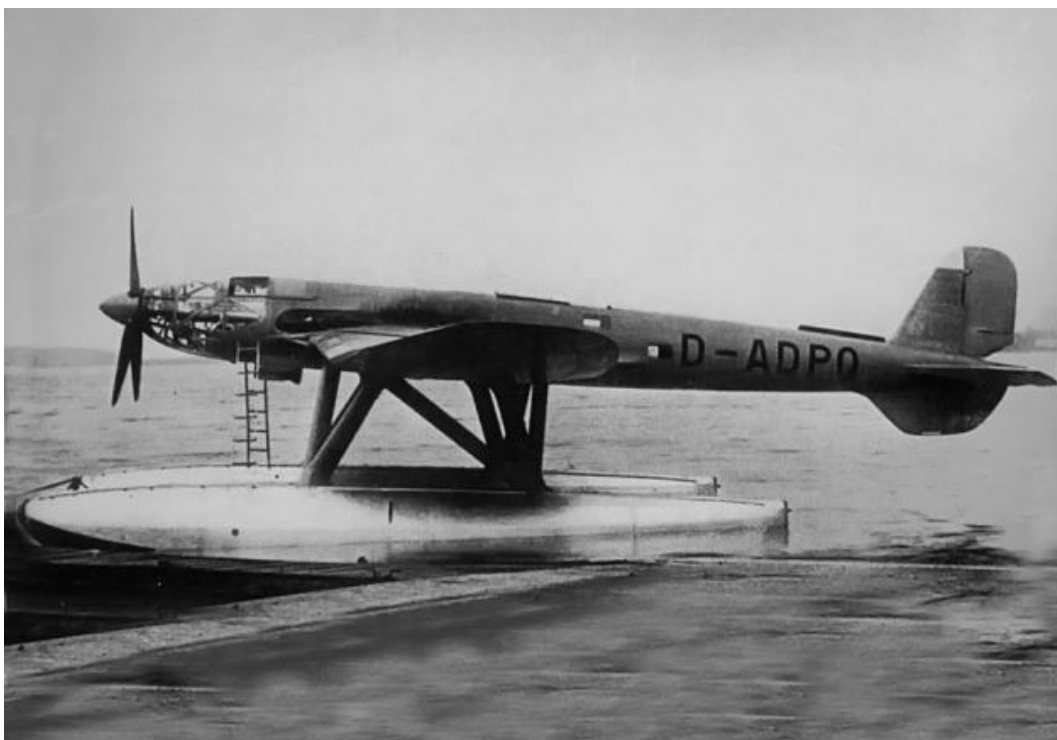
Side view of the He 119 V3. The updated wing used on the V3 and all further He 119 aircraft can be seen as well as tail modifications to increase the seaplane's stability.
