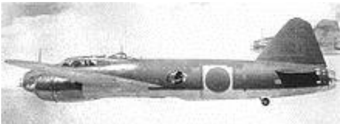
A Mitsubishi G4M1; with a non-standard roundel - a white square instead of the white circle surrounding the hinomaru .
