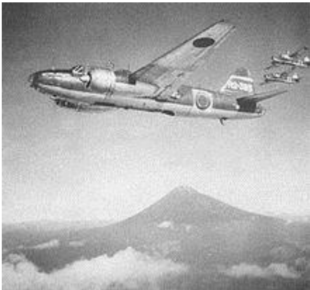
Mid- or late-production G4M1 Model 11s with the propeller spinners and rubber ply beneath the wing fuel tanks.
