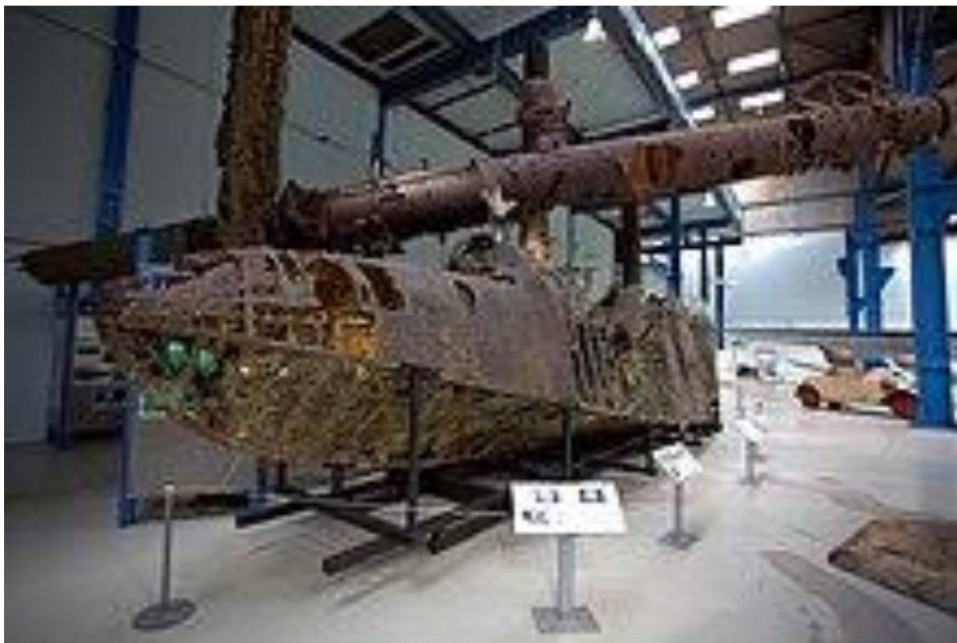
The wreck of NJ+HE a Blohm & Voss BV 138 at display at the National Museum of Science and Technology (Danmarks Tekniske Museum) in Elsinore, Denmark. The wing spar is poised over the aircraft in the same position as it was, when the wreck was discovered in The Sound, off Copenhagen.
