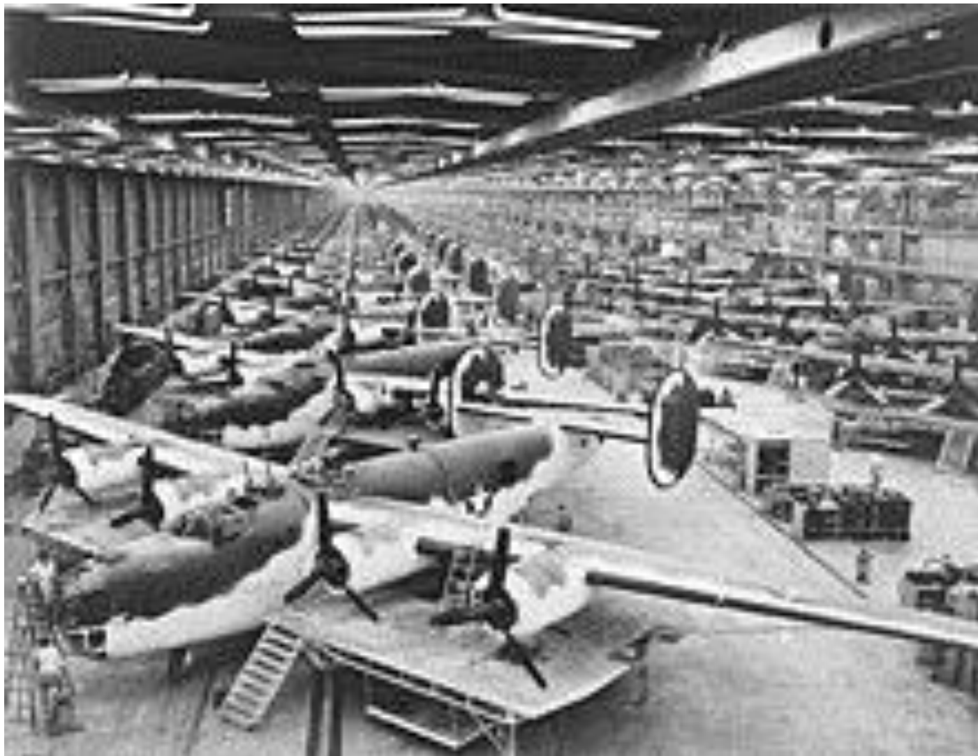
AAF Antisubmarine Command (AAFAC) modifications at the Consolidated-Vultee Plant, Fort Worth, Texas in the foreground in the olive drab and white paint scheme. To the rear of this front line are partly assembled C-87 "Liberator Express Transports"
