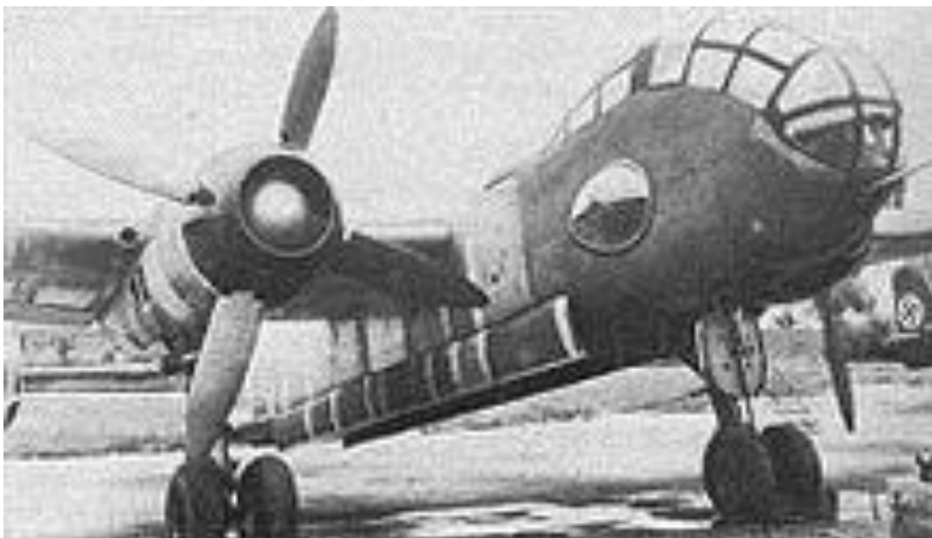
A Jumo 222-powered Junkers Ju 288 prototype with ducted spinners, of a similar type to that intended for the Ar 240.
