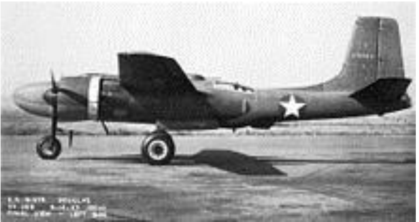
Douglas XA-26B Invader AAF Ser. No. 41-19588, 5 May 1943, with a "strafer" nose, was adaptable to a combination of weapons, including a 75 mm (3 in) cannon.
